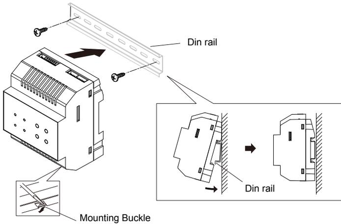
Step1: Mount the din rail to the wall with screws ;
